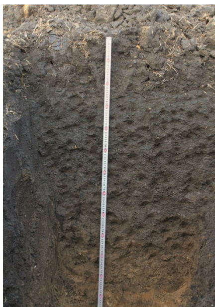
Photo 1. Karasoluk – heavy clay . Vertic Chernozems v. Primortsi Photo 2. Slightly leached Chernozem –Haplic Chernozem. v.Vetrino Fig.7 – Profiles of Chernozems
